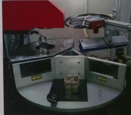
PW gets part type from plc. Checks correct part type by read RF id tag on pallet. Nests are unique to part type. Sends file to laser; triggers laser; mark complete; rotates turntable; fires camera to verify quality; sends results back to PW
