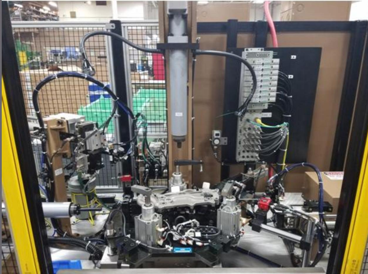
As the machine processes, all of the data from the torque guns and presses is recorded. By the time an assembly is completed there will be in excess of 100 pieces of information associated with the part.
