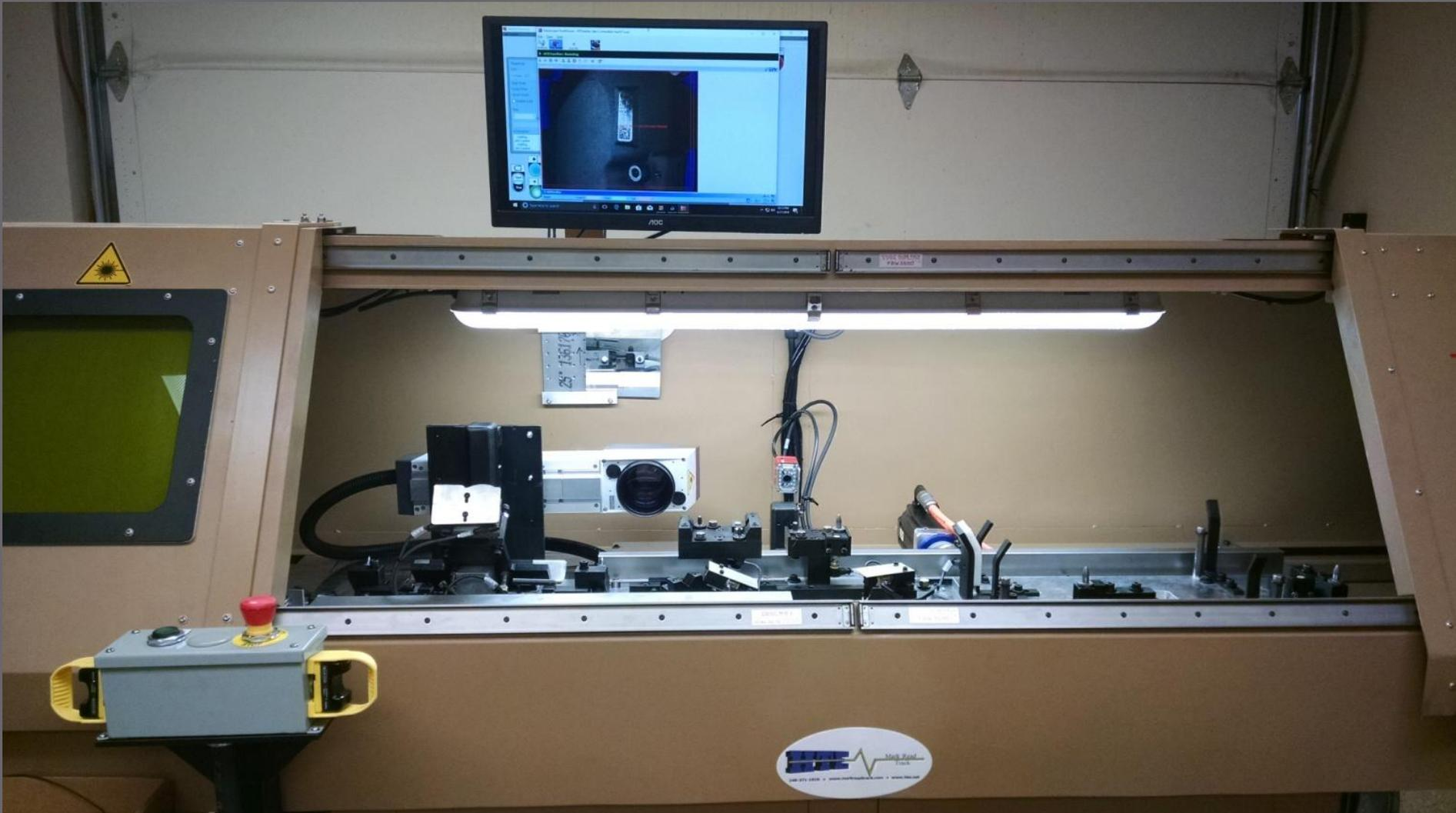
After the parts are marked they are checked for good mark quality and decode content. Each part is uniquely identified and the data associated with the part is logged to Plantwatch. Later this data will be used to verify that the mark quality was good before any work is done with the part.
