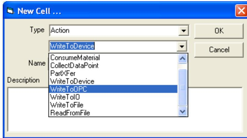
After accepting the base configuration of the cell, open the cell and you will be able to select the OPC server and enter the address the information is written to, as well as what is to be written.
