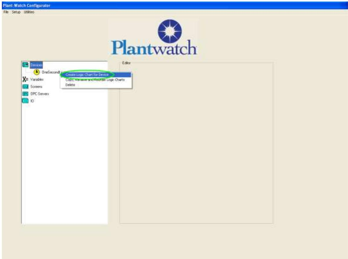
Right click on our new device *OneSecondInterval* and select *Create Logic Chart For Device*. You will be presented with the dialog to name and create a new logic chart.
