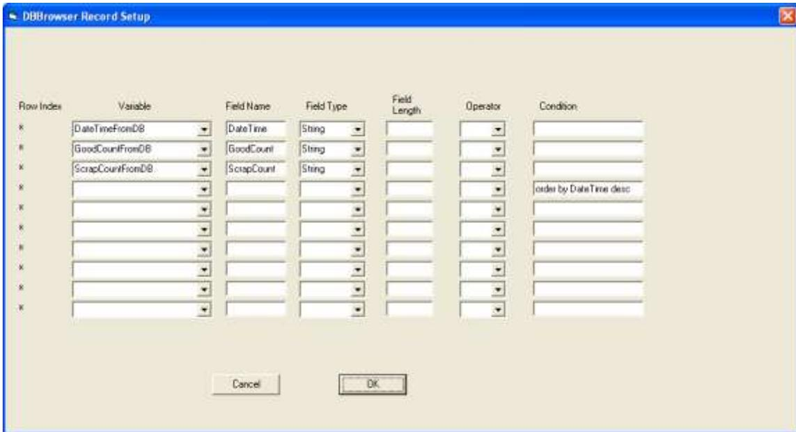
This configuration has a Condition field populated in a row that has no field or variable selected. In this case DBBrowser will simply attach the string onto the end of the Select. This allows significant flexibility in what DBBrowser can do
