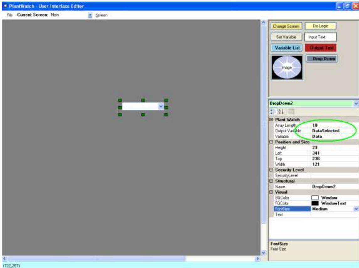
This animation type has a setting for the security level needed to invoke the action. If left blank then no security is applied.
