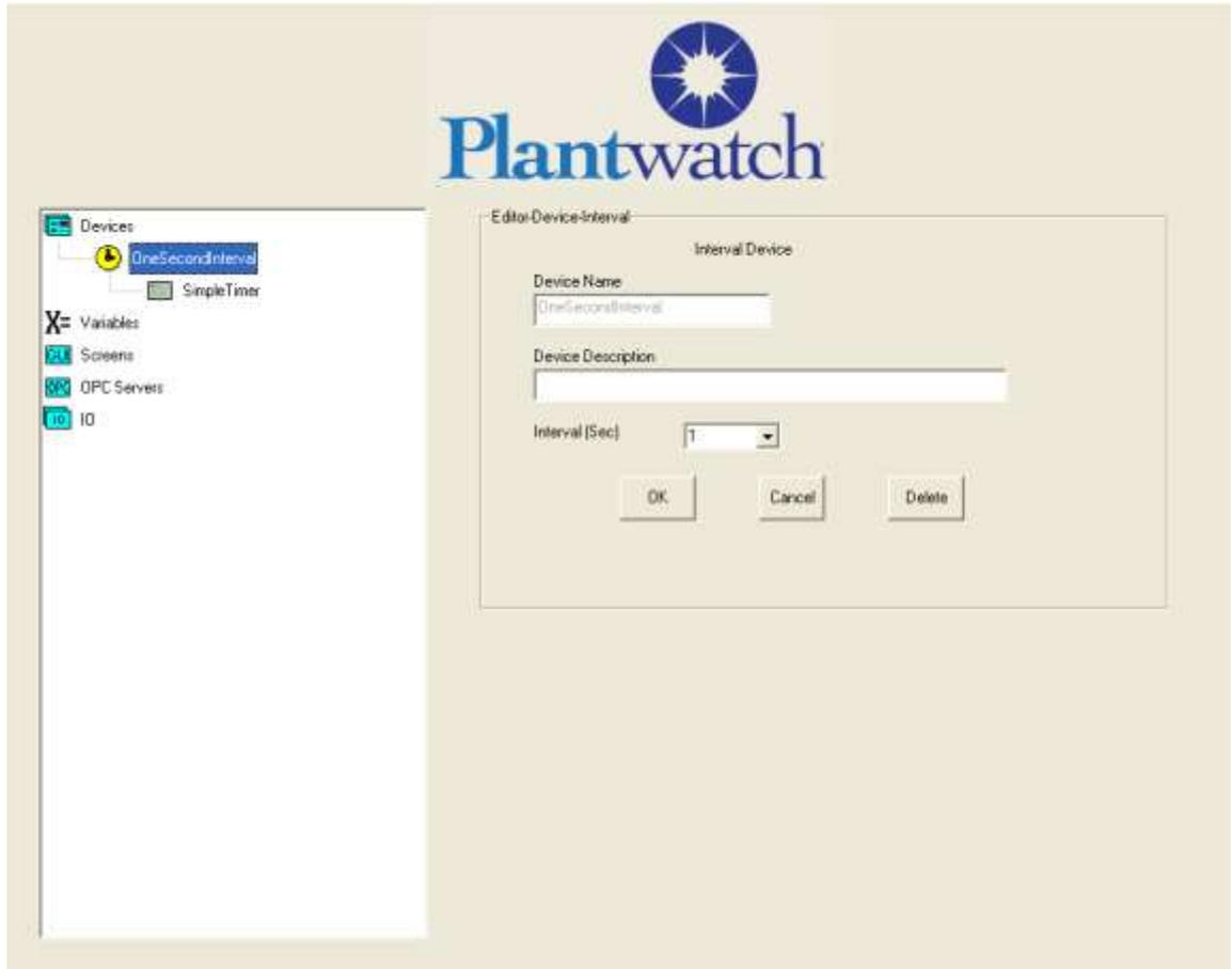
When you expand out devices you will see our device *OneSecondInterval*. You can now expand our device to see our new logic chart called *SimpleTimer*
