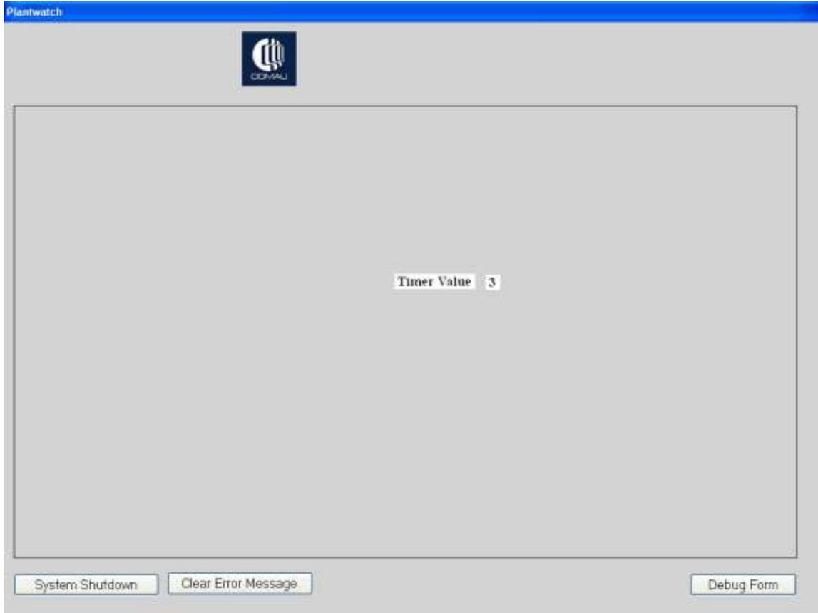
To shut off *PlantWatch Runtime* select the *System Shutdown* button, enter the password and then select the *Shutdown* button. Default password is 123.
