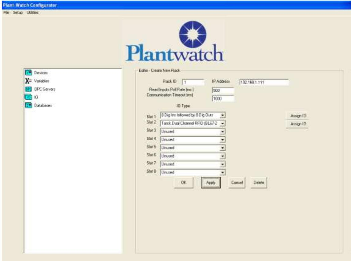
For each input card there will be associated Assign IO button. Select this button to assign variables to each of the input points. Prior to assigning the variable you must first have created the variables.
