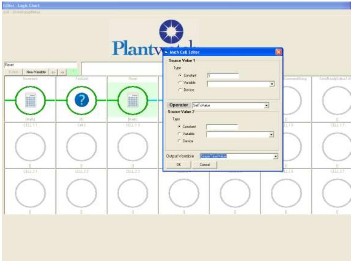
Double click on the third cell to configure the reset logic. We will use a math cell to set our counter, variable SimpleTimerValue, to one.
