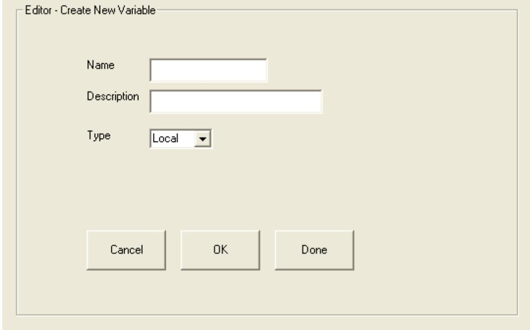
Enter a name and description, and then change the *Type* from *Local* to *Array*. You will see a new field appear for you to configure called *Array Length*. The example below shows an Array Type Variable three long called Data being created.
