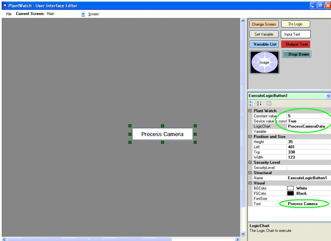
Settings to execute Logic Chart *ProcessCameraData* with a constant device value of 5
