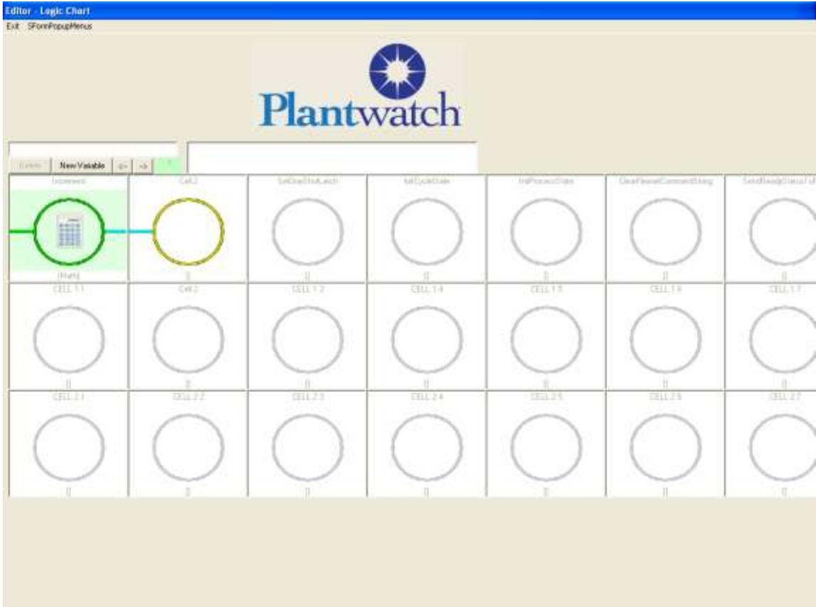
Now the upper left cell is displaying the Math cell icon, a calculator. Note that the second cell is available for use. Double click on the math cell to set it's configuration.
