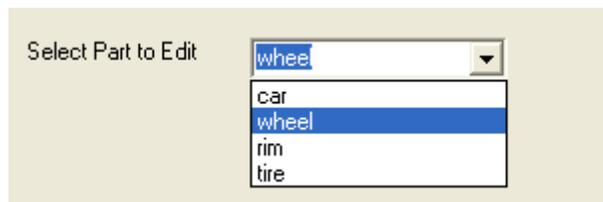
To configure our wheel to be made of a rim and a tire we will first select it in the *Select Part To Edit* list box, and then we will select the *Add Sub Part Number* button.
