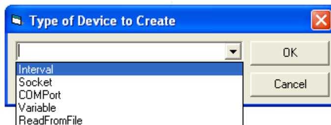
Select *Interval* from the list and then select *OK*. You will be presented with the configuration panel for an Interval type device.
