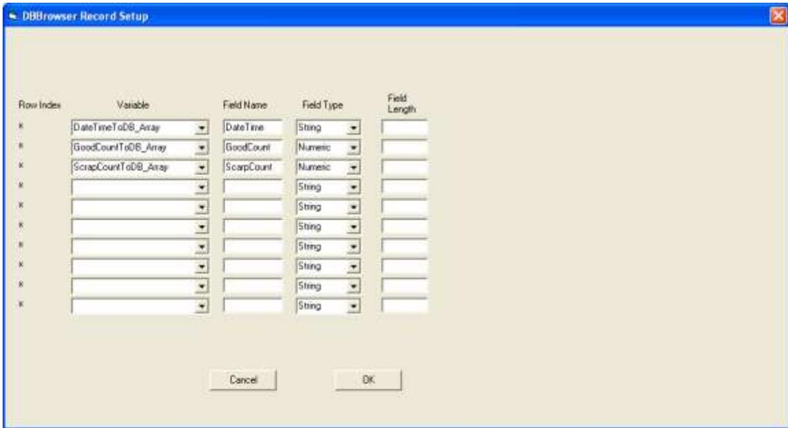
The second level configuration with Arrays is the same as not using Arrays. The difference now is that 5 inserts will occur.
