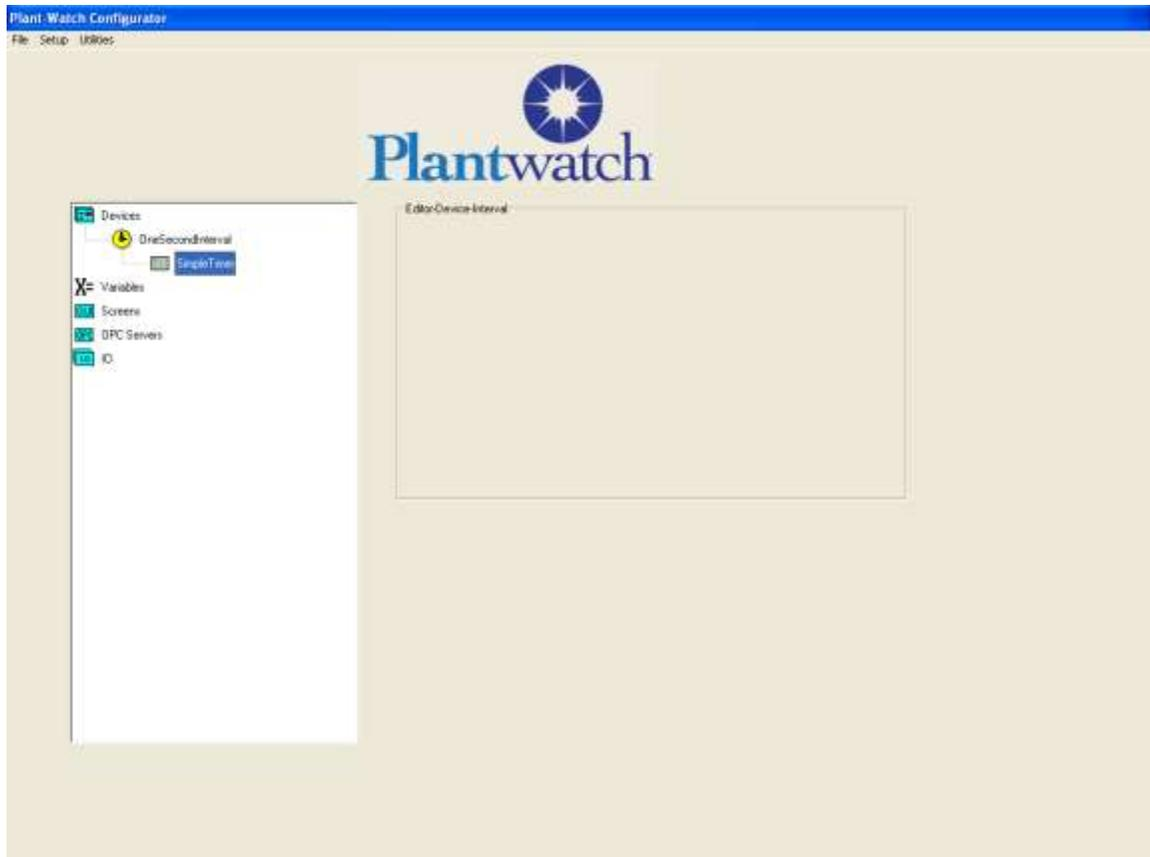
To Define our Logic Chart SimpleTimer, expand out devices by double clicking on Devices.
